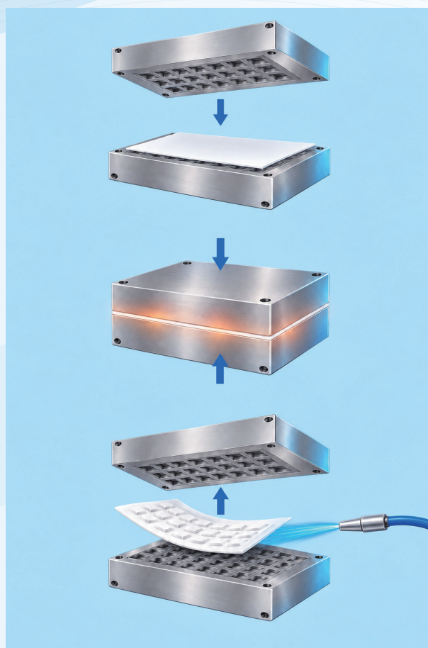
Placement · Curing · Release
